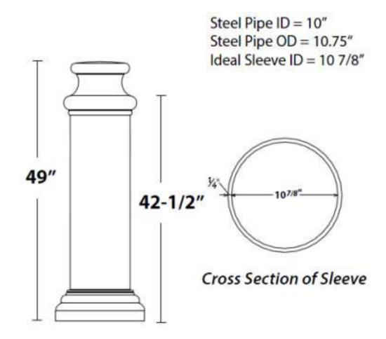
Made of: 1/4" nominal wall thickness polyethylene plastic Colors: Available in any color to match corporate branding Installation: 2 pieces of patented installation included per bollard cover
