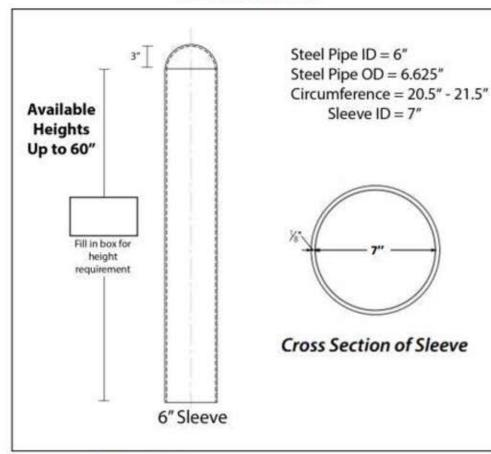
Made of: 1/8" nominal wall thickness polyethylene plastic
